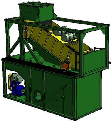
The pump tank module consists of a heavy duty hollow section steel frame which houses a tank into which the shaker underflow falls and 2 No. Metso MM200 centrifugal pumps each with overhead mounted 45kW motors and star-delta starting. These pumps are used to discharge the screened fluid from the SD1000DP to downstream equipment, such as SM500PSDP units for finer cleaning.
